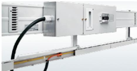
The tap-off/ancillary equipment unit combination is networked via the AS-Interface and facilitates remote monitoring/switching.
